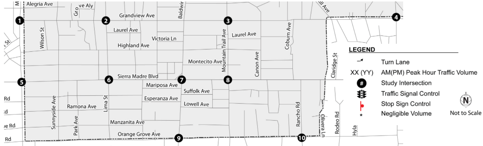
Figure 3-3a Existing Intersection Lane Configurations and Peak Hour Traffic Volumes
